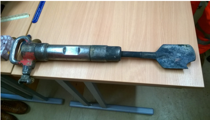
(Damage to clay spade)
