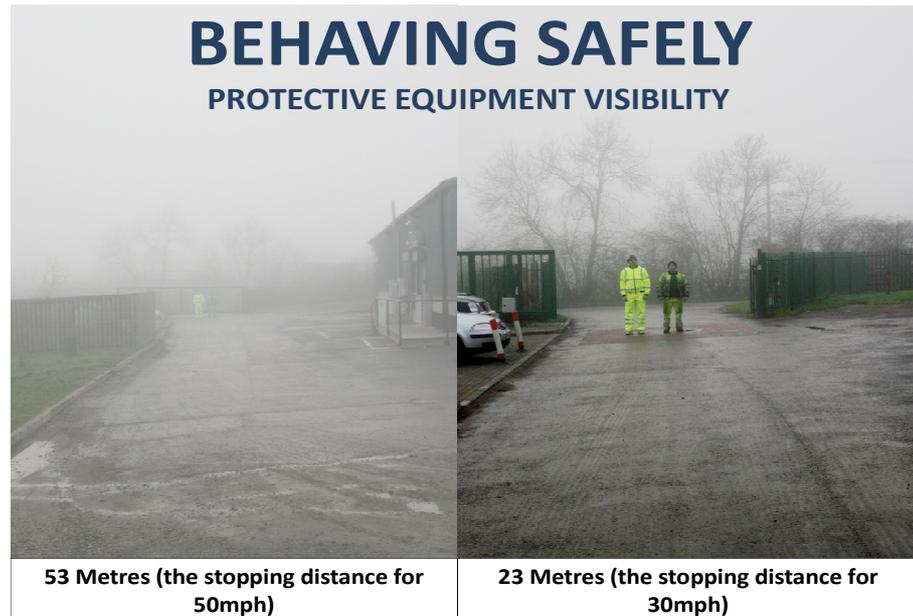
**The operative to the right in the picture on the left is not visible at 53 metres. Therefore not giving the driver of the vehicle enough time to stop at 50mph.**
