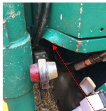
Damage sustained to chassis and steel winch wire thimble
