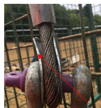
Damage sustained to chassis and steel winch wire thimble
