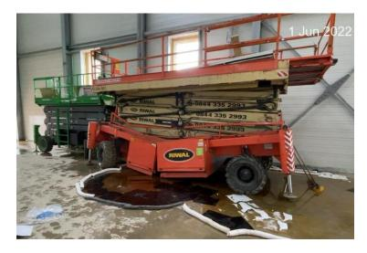
The type of MEWP involved is a **Holland Lift Model type: HOL-M250DI27**, a fitter from the rental company and manufacture are on their way to site to undertake a technical investigation. SE GP T HG will also complete an investigation as required by internal procedures and findings from both will be made known as soon as possible.
