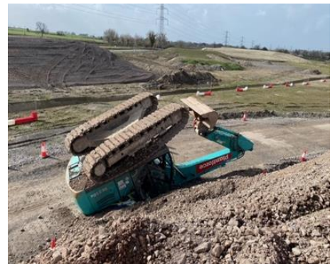
Overturned excavator in final resting position at foot of stockpile.
