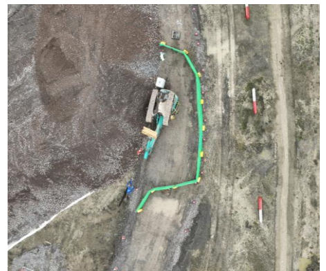
Overturned excavator in final resting position at foot of stockpile.
