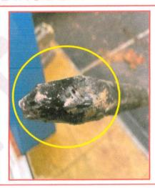
An incident recently occurred on one of our developments when a landscaping operative struck a live buried HV electric service with a steel digging bar, as shown above.
