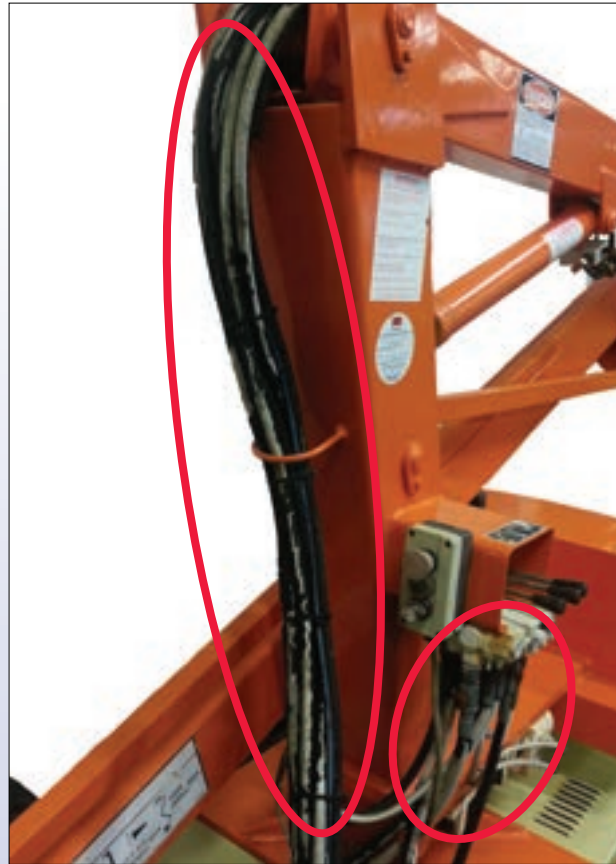
Damage along almost the full length of each hose assembly
