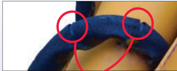
Hose burst sleeve split
