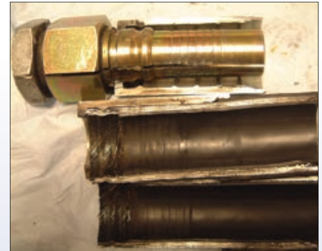
The above photograph shows radial cracks in the hose liner
