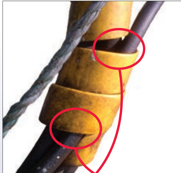
The hose is trapped within the spiral wrap
