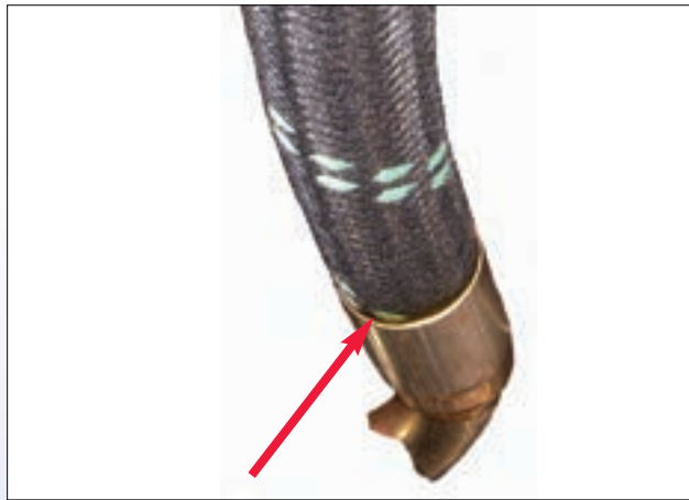
Witness of oil which shows on the hose cover
