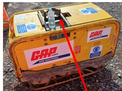
Single lifting point in raised position to enable lifting by other plant
