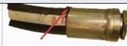
Hose cover extruding out of the ferrule
