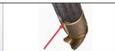
Witness of oil which shows on the hose cover
