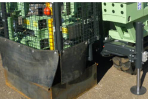
Above: Rubber infill used to extend guard down and accomodate flush system.
