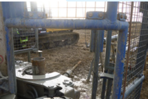
Above: Large, unnecessary gap that permits access to dangerous parts.
